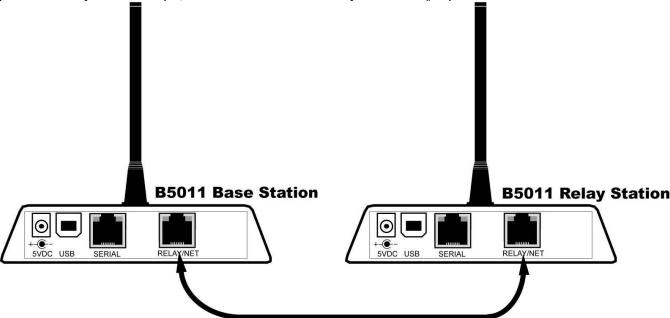
To add additional Relays, you must "multi-drop" them off a single bus line running from the "RELAY/NET" port on the Base station. See the section below for cabling requirements and pin-outs. It is very important to follow the pin-out directions carefully and to use the suggested cable type. The majority of problems we see are the result of incorrect wiring.
