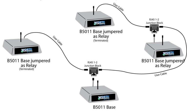
Notice that the two end units are terminated; the units in the middle are unterminated, including the Base in this example. Keep in mind that the maximum total cable length from end-to-end is 4000' for good quality twisted pair wire.
