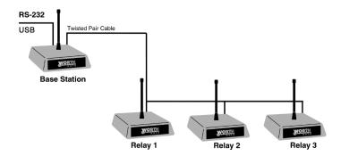
Relay Stations are attached to the Base Station using a cable that connects from the Base's RELAY/NET port to the Relays' RE-LAY/NET port. When you order a Relay Station, you receive a short test cable with it. Although Relay Stations will increase your range of operation, they will also add about ½ second to the response time.
