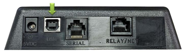
You need to connect to a full power USB port (0.5A) typically these are the motherboard connectors on a desktop computer. You will need a power supply if you are connected to a low power USB. Many laptops, all-in-one computers, and some of the newer micro form factor computers may only have low power USB ports. A powered USB hub will also work in those situations.
