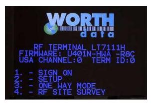
On second line on the screen, FIRMWARE: Uxxx, gives the firmware revision number. The letter U indicates USA frequency. Rzz refers to the version of the radio processor firmware.
