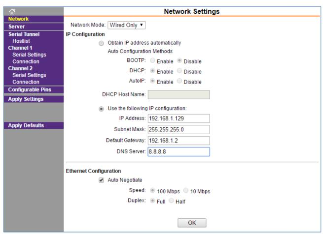
In this example the IP address of the Base is set to 192.168.1.129. Yours will probably be different but you will need to know the IP address of the Base to set up the Relays. The Gateway and DNS Server are not used for Option #2 networks since all Relays are located on the same LAN. If you change any settings click on "OK" before leaving the page to save the changes.
