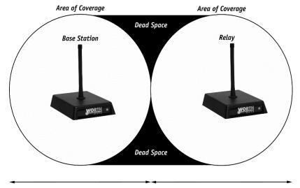
To Site Survey a Relay, all other Relays and Base Stations must be turned off. This is the only way to know for sure which Relay is responding. Alternatively, perform the Relays' test out of range of the other Relays and Base Stations.
